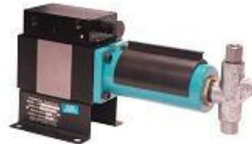
This low-consumption unit can run either air or gas. The inlet pressure ranges from a minimum of three psi (0.206 bar) to a maximum of 150 psi (10.342 bar). The choice of three plunger sizes, coupled with controllable strokes per minute (SPM) and a slow speed controller allows for a capacity ranging from less than 1 quart up to 60 gallons/day. This is a lightweight, reliable and rugged pump that can be serviced easily in the field.
